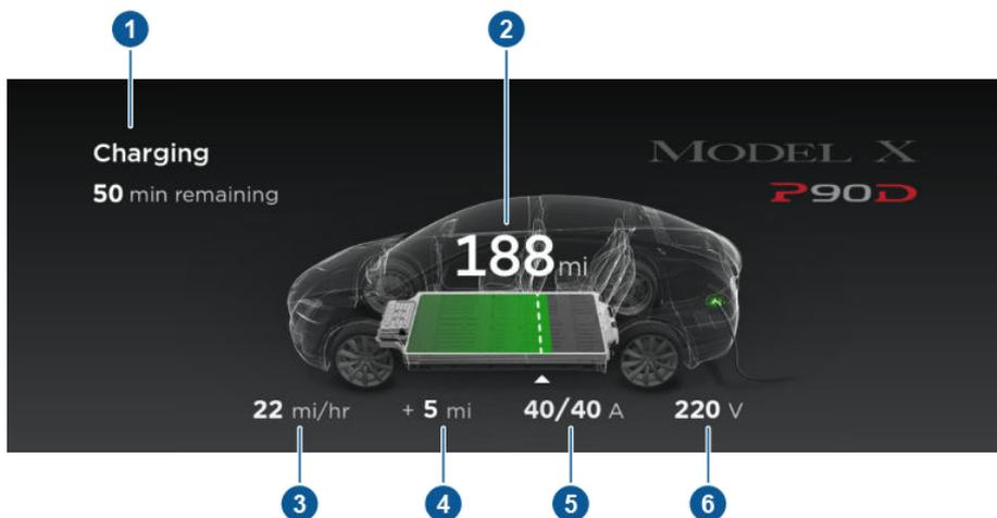
1. Charging status information. For example, when Model X is charging, it displays the time remaining until fully charged at the currently selected charge level. When a charging session is scheduled, it displays when charging starts.
