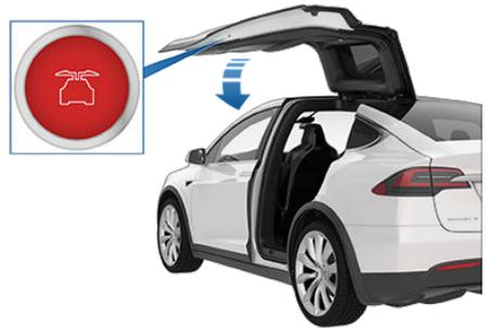
**Note:** To prevent children from opening falcon wing doors using the interior switch, turn on child-protection locks using the touchscreen (**Controls > Vehicle > Child- Protection Lock**). See [Child-Protection Lock](#) on page 17.
