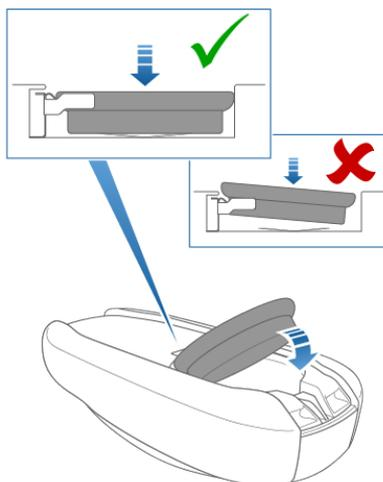
**Note:** Wipe the battery clean before fitting and avoid touching the battery's flat surfaces. Finger marks on the flat surfaces of the battery can reduce battery life.
