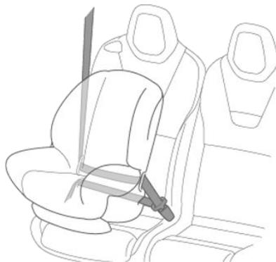
2. Allow the seat belt to retract, and remove all slack in the seat belt while firmly pushing the child safety seat into the Model X seat.
