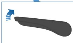
**Warning:** Riding in a moving vehicle with the seat back reclined can result in serious injuries in a collision, as you could slide under the lap belt or be propelled into the seat belt. Ensure the backs of occupied seats are reclined no more than 30 degrees when the vehicle is moving.
