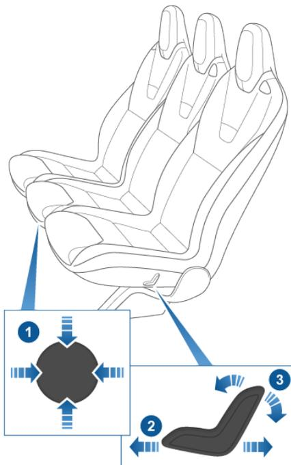
1. Move seat forward/backward (up/down on the control) and adjust the backrest (left/right on the control).
