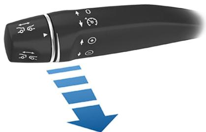
After setting the cruising speed, release the accelerator pedal to allow Traffic-Aware Cruise Control to maintain your set speed.
