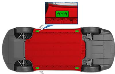
5. Adjust the height and position of the lift arm pads to ensure that they are correctly located.
