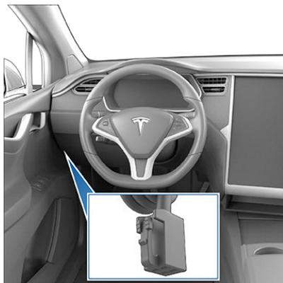
4. Connect the pigtail connector to the vehicle wiring connector.
