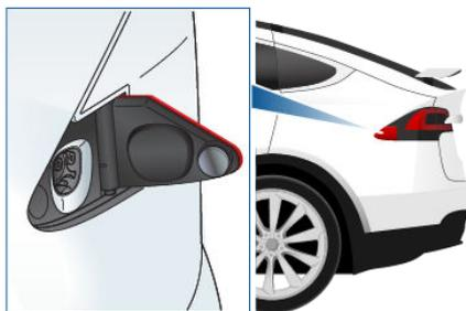
**Note:** The charge port lights up white when you open the charge port door. If you do not insert a charge cable into the charge port within a few minutes after opening the charge
