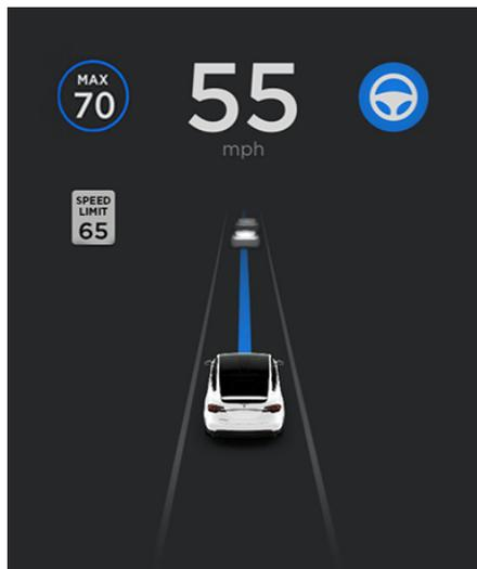
When Navigate on Autopilot is active and you approach an off-ramp or freeway interchange along your navigation route, the appropriate turn signal engages and Autosteer maneuvers Model X onto the off-ramp or interchange.
