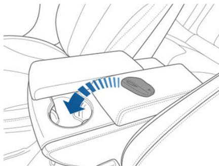
If Model X still does not detect the key, try holding it against the center console, immediately below the 12V power socket (see [12V Power Socket](#) on page 25). If the key is still not detected, remove the key's battery and try again. See [Replacing the Key Battery](#) on page 11. Or try using another key. If another key does not work, contact Tesla.
