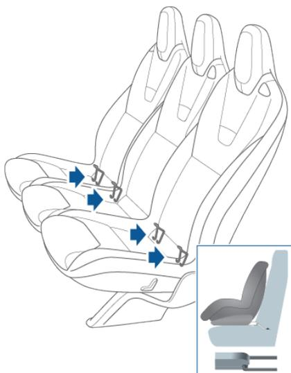
Once installed, test the security of the installation before seating a child. Attempt to twist the child safety seat from side to side and try to pull it away from the seat, then check to ensure the anchors remain securely in place.
