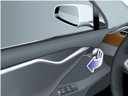
You can also use the touchscreen to open and close doors when inside Model X. Touch **Controls > Quick Controls**, then choose the door you want to open or close. In addition, if Model X is equipped with the premium upgrades package, when you press the brake pedal, the driver's door automatically closes.
