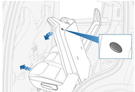
**Warning:** For vehicles with third row seats, do not use the third row ingress button located on the backrest of a second row outboard bench seat when a child is seated in the second row. Using the button allows the combined left and center seats to be moved forward and can squeeze the occupant. Use this button only when the second row seats are unoccupied. Before driving, ensure the seat and the seat back are securely latched into position.
