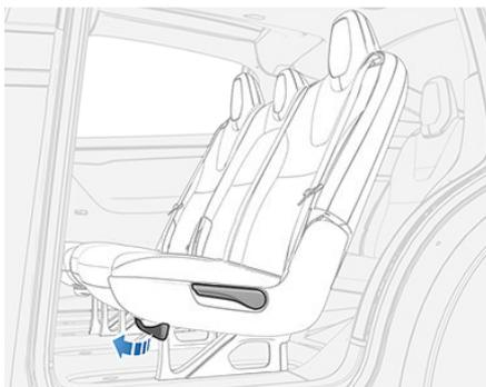
**Note:** You can adjust the position of bench seats using the mechanical levers only. You cannot use the touchscreen to adjust bench seats.
