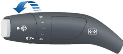
For a single wipe, press and release the end of the lever.
