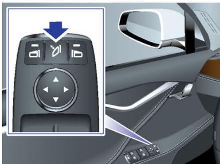
The driver's side mirror automatically dims at night, in proportion to the level of glare from the headlights of a vehicle behind you (except when in Reverse gear). Also, both exterior side mirrors have heaters that turn on and off with the rear window defroster.
