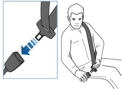
4. Pull the belt to check that it is securely fastened.
