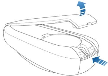
**Note:** If a lanyard is attached to the key, you can release the bottom cover by placing your thumb against the "X" on the bottom cover, then firmly pulling the lanyard toward you (hence pushing the key off of its cover). You can also pry the cover off by placing a small flat-bladed tool, a fingernail, or the Tesla-provided tool against the lanyard cord.
