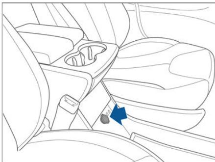
The 12V power sockets are suitable for accessories requiring up to 11A continuous draw (15A peak) or a maximum of 150 continuous watts (180 watts peak).
