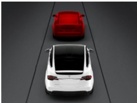
Warnings cancel automatically when the risk of a collision has been reduced (for example, you have decelerated or stopped Model X, or the object in front of your vehicle has moved out of your driving path).
