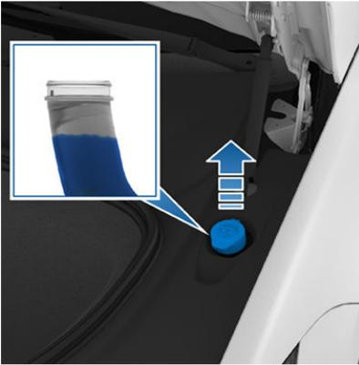
4. While avoiding spilling, fill the reservoir until the fluid level is visible just below the filler neck. The reservoir has a capacity of liters.
