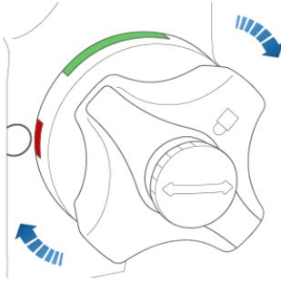
**⚠ Warning:** Be careful when turning the locking cylinder. If it does not lock into the "Open Position", it automatically retracts into its original "Closed Position" and can pinch your fingers.
