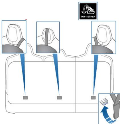
For single-strap tethers, position the strap in the outboard seating positions over the outside-facing side of the head restraint (the same side of the head restraint as the seat belt retraction mechanism). In the center seating position (if equipped), center and position the strap over the top of the head restraint.
