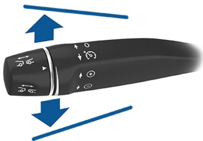
**Note:** When Traffic-Aware Cruise Control cancels, Model X does not coast. Instead, regenerative braking slows down Model X in the same way as when you move your foot off the accelerator when driving without Traffic-Aware Cruise Control (see [Regenerative Braking](#) on page 77).
