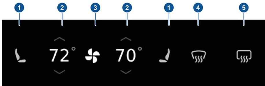
1. Seat heaters operate at three setting levels from 3 (highest) to 1 (lowest). When operating, the associated seat icon displays twisting lines that turn red to indicate the setting level. If equipped with ventilated seats, a popup appears that allows you to switch between heating and cooling. When cooling, the twisting lines turn blue.
