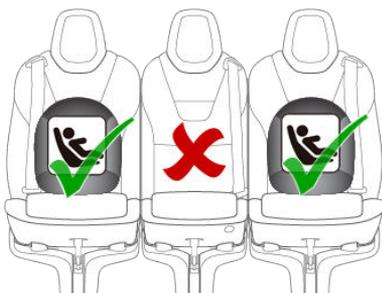
**Note:** To accommodate large rear-facing LATCH child safety seats, you may need to move the seat in the full rearward position, and move the corresponding front seat forward to the mid-track position (up to 13 cm forward of the rearmost position), raise the seat upward (3 cm from its lowest position), and angle the seat back to 15 degrees (or 10
