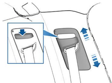
3. Release the button on the shoulder anchor so that it locks into position.
