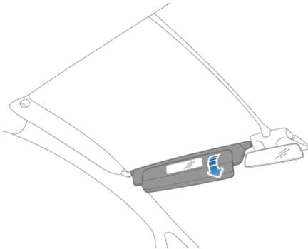
To protect front seat occupants from sunlight coming through the side window, lower the sun visor from the pillar then lower the visor extender.
