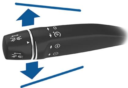
To set the cruising speed to the speed limit plus any offset you've specified using Speed Assist, pull the cruise control lever toward you. If you are already driving faster than the speed limit, the set speed does not adjust to the speed limit—it adjusts to your current driving speed. If you move the cruise control level up or down after setting Traffic-Aware Cruise Control to cruise at the speed limit, your set speed becomes your current driving speed.
