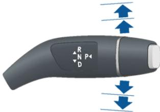
If you try to shift into a gear that the current driving speed prohibits, a chime sounds and the gear does not change.
