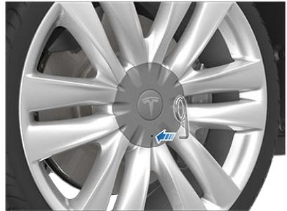
2. Maneuver the lug nut cover tool so that it is fully inserted into the hole in the lug nut cover.
