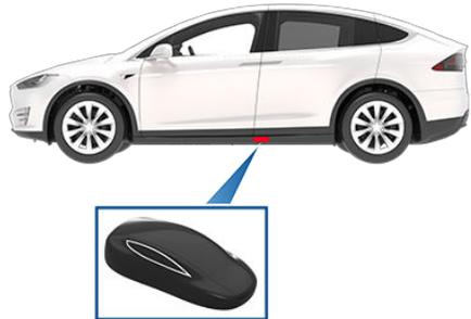
To drive Model X after gaining access to the cabin, place the bottom of the key against the center console, immediately below the 12V power outlet, then press and hold the brake pedal to start Model X.
