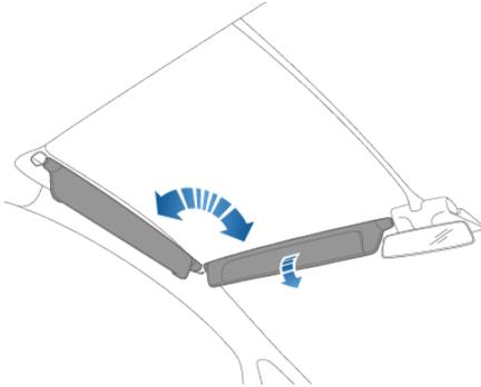
To expose the vanity mirror, lower the visor extender then lower the mirror cover. While the cover is lowered, the mirror is exposed and lights are illuminated.
