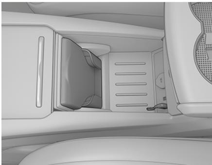
Model X will charge your smartphone only when the vehicle is powered on (i.e., the touchscreen is on and you are in the vehicle). Your smartphone will not continue to charge if you leave it plugged in after exiting the vehicle. Model X will not charge your smartphone if the vehicle's Battery is discharged.
