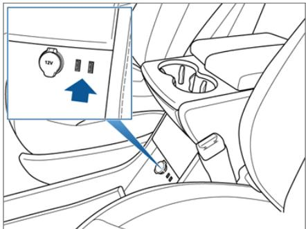
In addition, Model X has two charge-only USB ports located at the rear of the center console, and another charge-only connection located between the third row seats.
