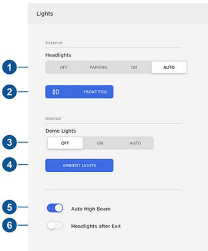
1. Exterior lights (headlights, tail lights, side marker lights, parking lights, and license plate lights) are set to **AUTO** each time you start Model X. When set to **AUTO**, exterior lights automatically turn on when driving in low lighting conditions. If you change to a different setting, lights always revert to **AUTO** on your next drive.
