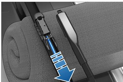
7. Fully insert the washer hose onto the nipple of the new wiper blade.
