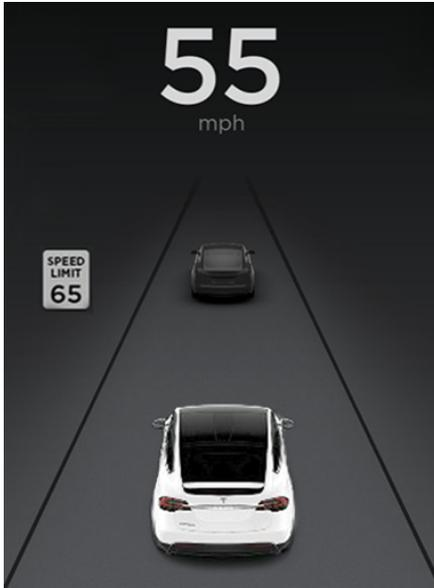
In situations where Model X is unable to determine a speed limit, or if Speed Assist is uncertain that an acquired speed limit is accurate, the instrument panel may not display a speed limit sign and warnings do not take effect.
