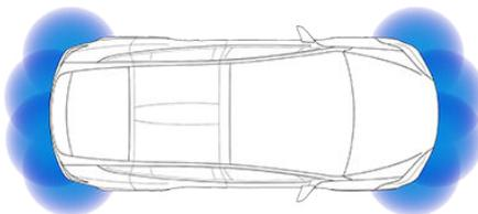
**Note:** Rear sensors are disabled when a bicycle is detected or Model X is in trailer mode.
